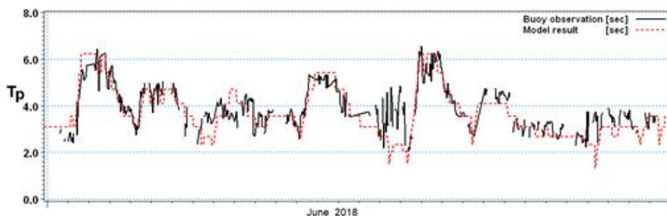
Figure 15. A comparison of measured wave peak period ( T_p ) with the simulated values in Booyeh, Asaluyeh during June 2018
