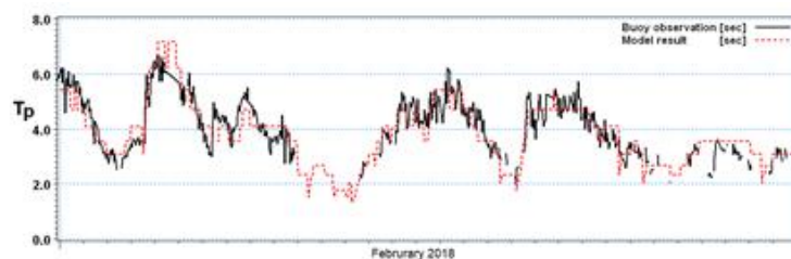
Figure 14. A comparison of measured wave peak period ( T_p ) with the simulated values in Booyeh, Asaluyeh during February 2018
